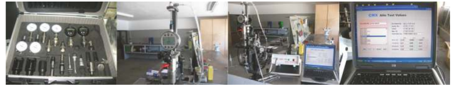
Cmx 108 SET OF SPECIAL TOOLS FOR DISASSEMBLING, ASSEMBLING AND MEASUREMENT OF BOSCH COMMON RAIL INJECTORS
